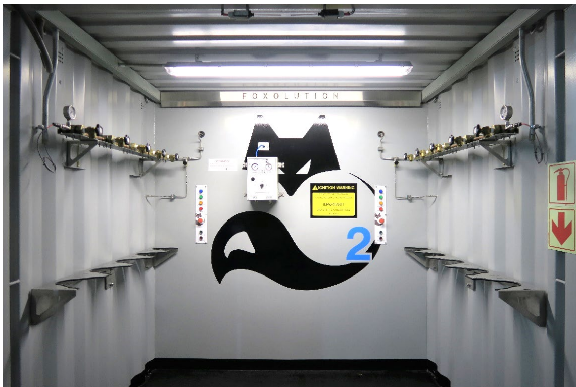
IMAGE 03: MEDFOX-100-CT 10-WAY CYLINDER FILLING CHAMBER WITH VACUUM STATION
