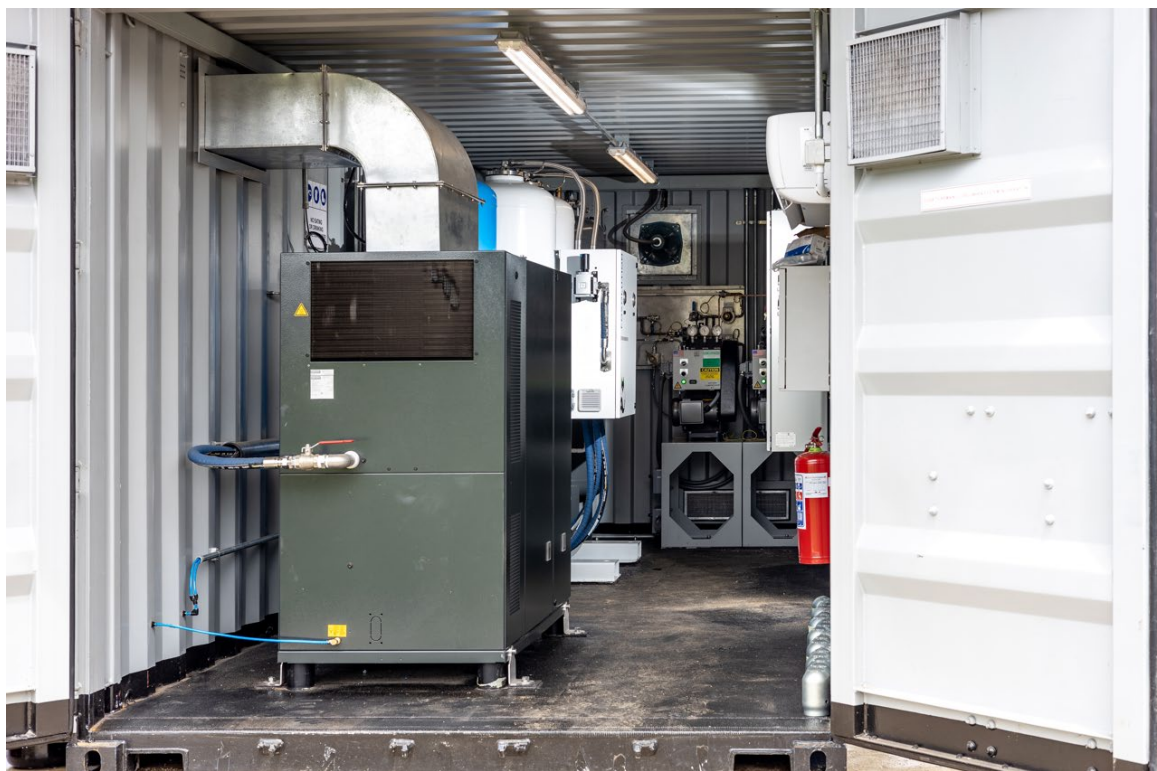
IMAGE 08: MEDFOX-185-CT-DS CONTAINERISED OXYGEN 93% CYLINDER FILLING SYSTEM INTERIOR
